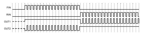
Fig.17 PWM control operation (timing chart)
