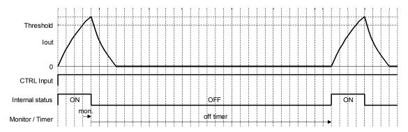
Fig.18 Over current protection (timing chart)
