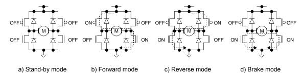
Fig.15 Four basic operations (output stage)
