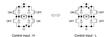
Fig.16 PWM control operation (output stage)
