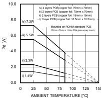
Fig.21 Thermal derating curve (HRP7 package)
